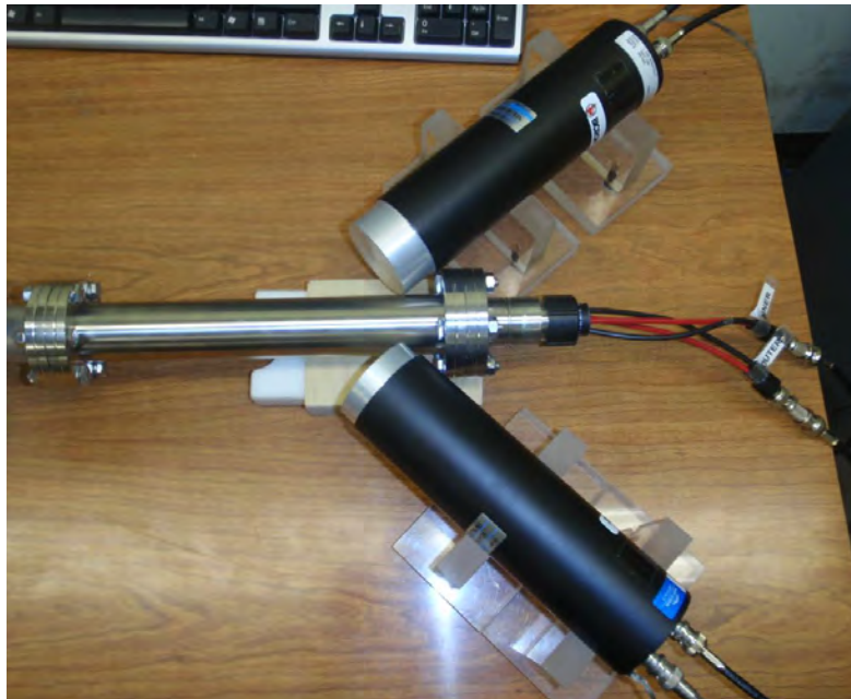
Figure 16. Capillary tube source system in vacuum chamber with while conducting lifetime measurements with BaF 2 detectors. At the right end of the tube the hookups for the applied electric fields can be seen.
