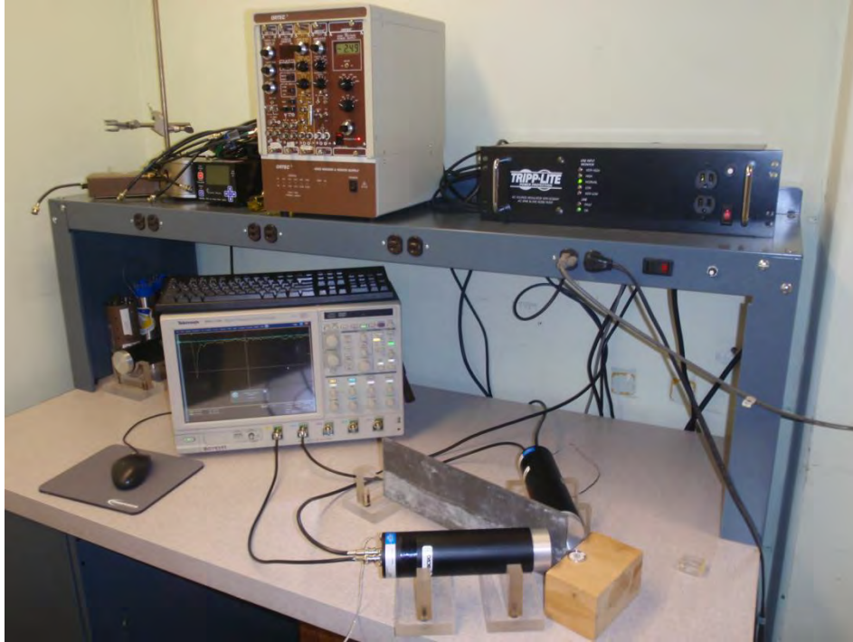
Figure 15. Positron lifetime spectroscopy setup
